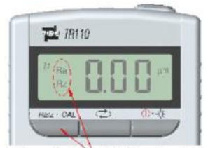
Ra/Rz conversion by press the Left Key gently and quickly
