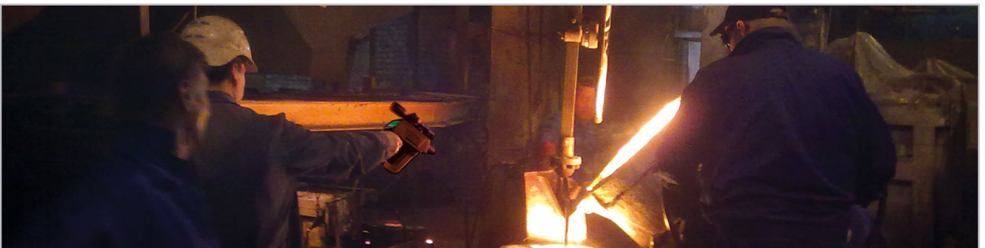
Non-contact temperature measurement from a safe distance
