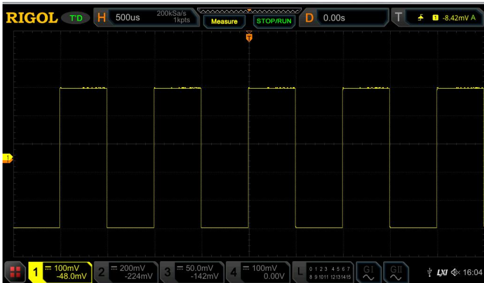
Figure 4-3 Waveforms after 128 Times of Averaging
