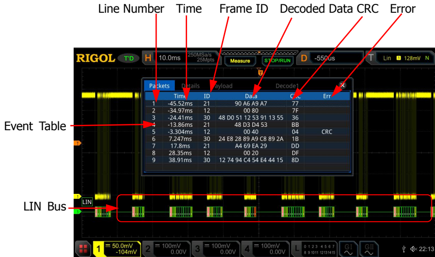
Figure 11-9 LIN Decoding Event Table
