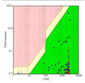
Tested at 5% dimming level.
