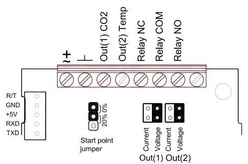
Terminals and jumpers on aSENSE GH (Disp) RL. Darker positions are default settings
