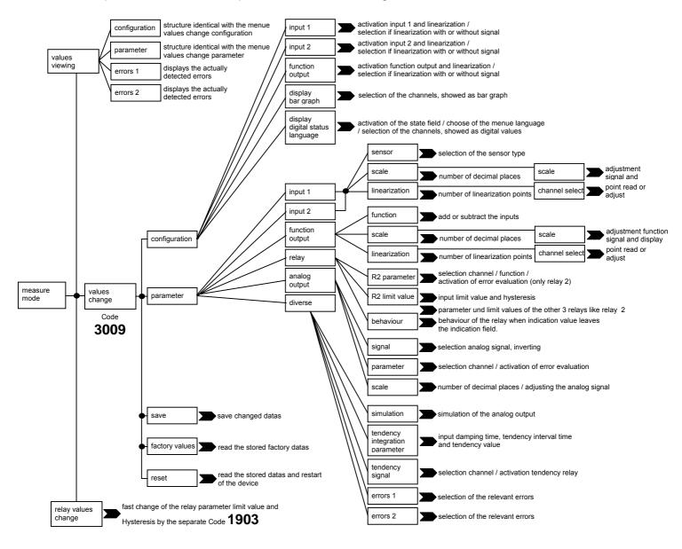
Use the key  ${\tt "OK}$ " to enter the **main menu**. From here **each menu** can be selected, using the keys  ${\tt "+}$ " or  ${\tt "-}$ " and entered, using the key  ${\tt "OK}$ ".
