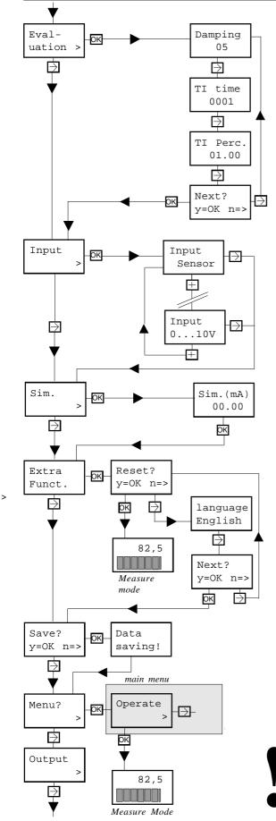
**Damping (integration-time):** In many using it is necessary to damp the outputsignal, especially when the level in a tank have been measured with large wave movements.
