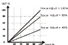
It's a scaling factor of the input command signal and limit the output of Thyristor unit. This parameter can be adjusted from 1 to 99% via RS485 or by the front of the unit. If this parameter is set at 50% and the input signal is 100% the output become 50%. This feature is very useful to reduce the power when a zone has been oversized or when a temperature controller gives same reference to more unit along a furnace.
