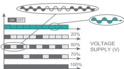
This firing is performed digitally within the thyristor unit at zero volts, producing no EMC interference. Analogue input is necessary for BF and the number of complete cycles must be specified for 50% power demand. This value can be between 1 and 255 complete cycles, determining the speed of firing. When 1 is specified, the firing mode becomes Single Cycle (SC).
