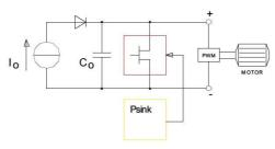
Power sink equipped power supply: absorbs breaking energy
