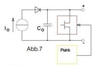
Power sink equipped power supply
