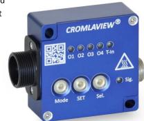
The sensor contains an own white light source clocked with a frequency of up to 2 kHz. Sampling takes place in both, the light and the dark phase. Additive ambient light cannot change the difference between the light and dark phase, so that the sensor is independent from ambient light.
