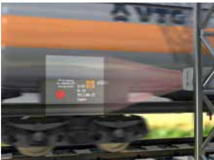
UIC wagon numbers and sign recognition CX cameras
