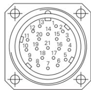
**Terminal assignment (connector 21-pin)**
