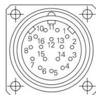
**Terminal assignment (connector 16-pin)**
