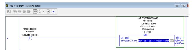
Double-click on question mark of "Output Unlatch" box. Select "Activate\_Preset" in the appearing drop-down menu. The result is shown below.
