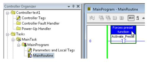
Type Ctrl+T to trigger a preset.
