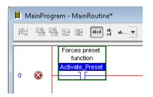
Double-click on question mark of "MSG" box. Select "Msg\_SET\_23\_13\_Preset\_Value" in the appearing dropdown menu. The result is shown below.
