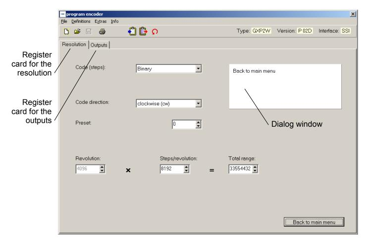
The parameters for the encoder can be set by means of the register cards for the resolution and the outputs. The dialog window gives additional support, or that is to say explains the window that has just been selected.
