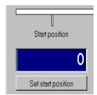
Bring the encoder to the desired start position by turning the encoder shaft. Enter the desired start value in the entry field start position, e.g. 0. Confirm entry by clicking "assign start position".
