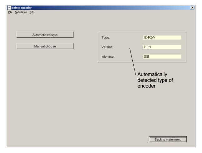
The type of encoder can be read out when the encoder is connected (automatic). This data is necessary to provide the relevant parameters for programming. If no encoder is connected or if the cable connection is not connected properly, an error message will be displayed. If the automatically detected encoder does not correspond with the encoder's type label, please contact Baumer IVO GmbH & Co. KG.
