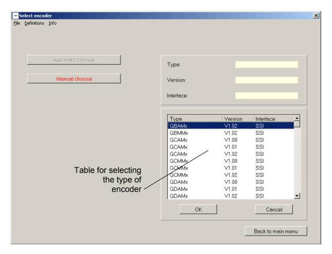
If no encoder is connected to the PC, the type of encoder can be selected from a table (manual selection). The table contains the common types. It is not only the type that is important but also the version. If your type should not be included, please contact Baumer IVO GmbH & Co. KG. Type and version can be found on the type label of the encoder.
