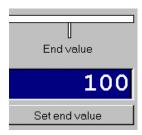
Thereupon bring encoder to the required end position and enter the desired end position, e.g. 100, in the field end position. Confirm entry by clicking "assign end position".
