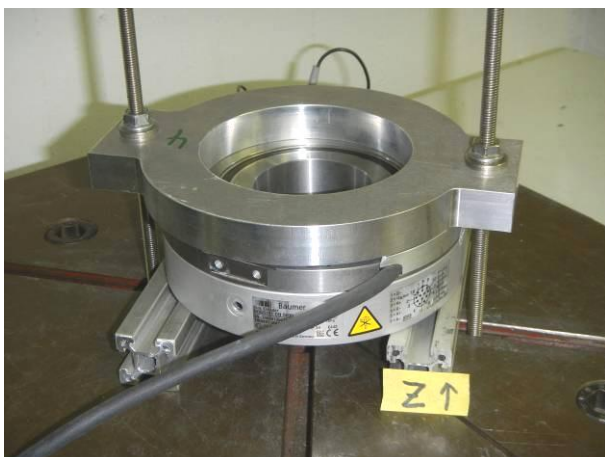
picture 11 Incremental Encoder HOGS 151 on the shock table with acceleration sensor during shock test in Z-axis, positive direction
