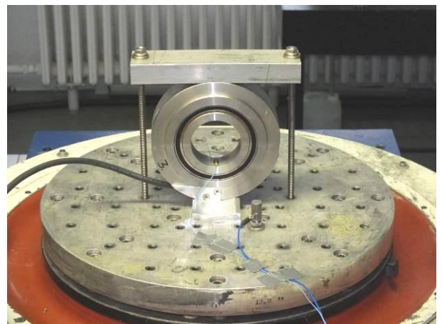
picture 4 Incremental Encoder HOGS 151 on the vibration table with acceleration sensors during vibration test in Y-axis
