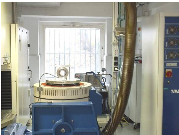
picture 3 Incremental Encoder HOGS 151 specimens on the vibration test device during vibration test in Y-axis
