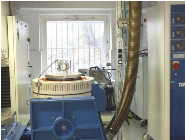
picture 1 Incremental Encoder HOGS 151 on the vibration test device during vibration test in X-axis
