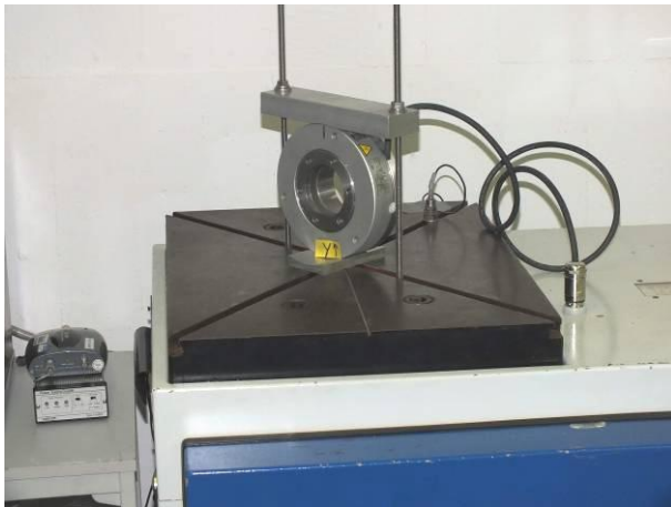
picture 9 Incremental Encoder HOGS 151 on the shock table with acceleration sensor during shock test in Y-axis, positive direction
