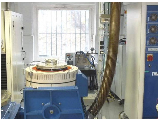
picture 5 Incremental Encoder HOGS 151 specimen on the vibration test device during vibration test in Z-axis
