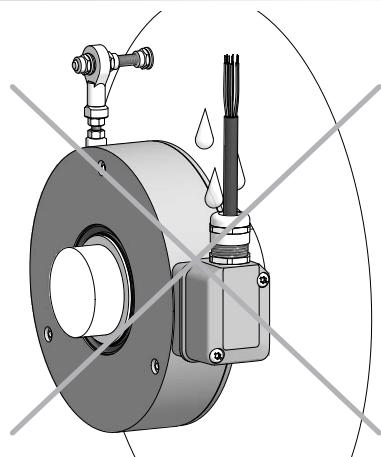
**i** It is recommended to mount the device with cable connection facing downward and being not exposed to water.
