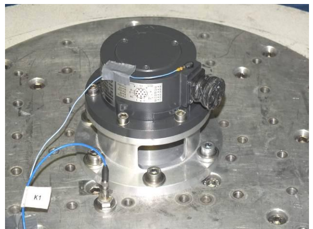
picture 6 Incremental Encoder FOG 9 on the vibration table with acceleration sensors during vibration test and shock test in Z-axis
