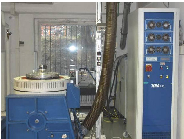
picture 5 Incremental Encoder FOG 9 specimen on the vibration test device during vibration test and shock test in Z-axis
