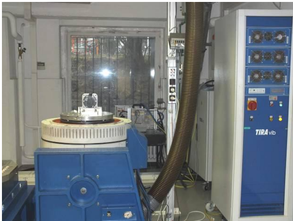
picture 3 Incremental Encoder FOG 9 specimens on the vibration test device during vibration test and shock test in Y-axis
