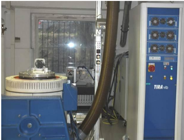
picture 1 Incremental Encoder FOG 9 on the vibration test device during vibration test and shock test in X-axis
