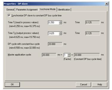
Time To is insignificant to the encoder. Usually the projecting software makes a proposal under consideration of correlations to other bus parameters.
