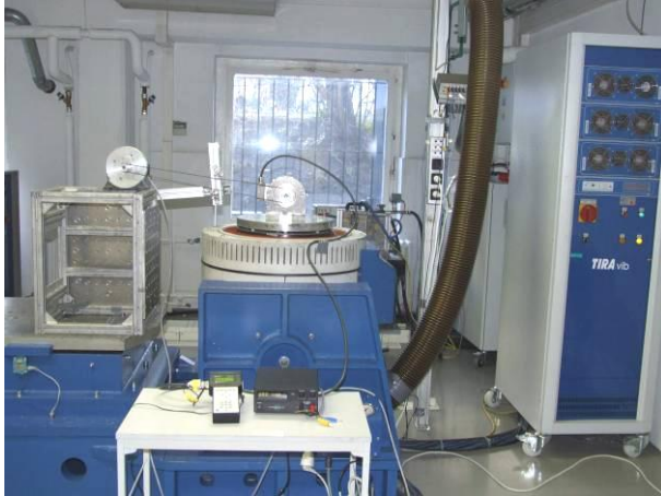
picture 1 Incremental Encoder HOG 165C on the vibration test device during vibration test in X-axis
