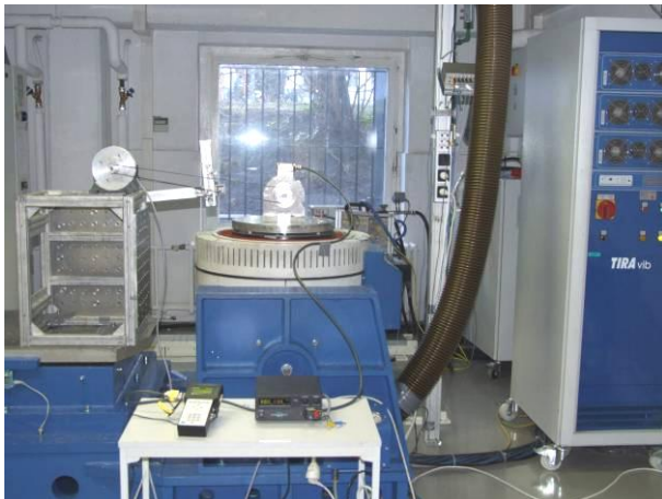
picture 3 Incremental Encoder HOG 165C specimens on the vibration test device during vibration test in Y-axis
