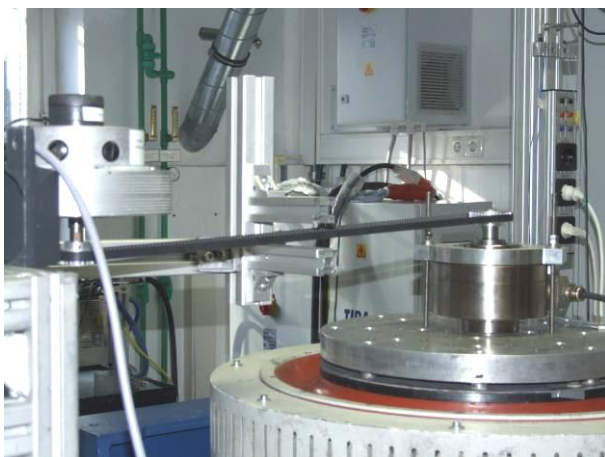
picture 5 Incremental Encoder HOG 165C specimen on the vibration test device during vibration test in Z-axis
