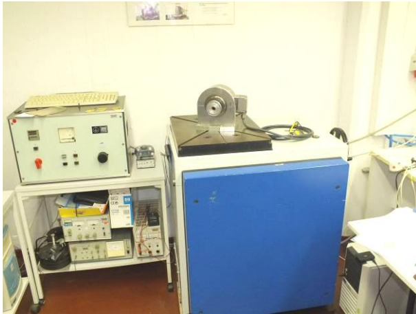
picture 7 Incremental Encoder HOG 165C on the shock table with acceleration sensor during shock test in X-axis, positive direction
