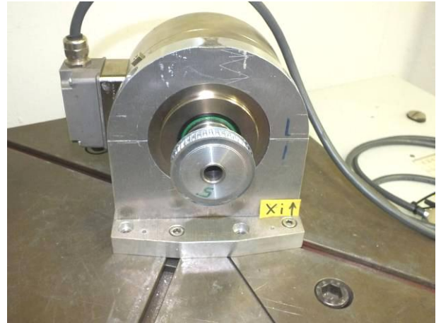
picture 8 Incremental Encoder HOG 165C on the shock table with acceleration sensor during and shock test in X-axis, negative direction
