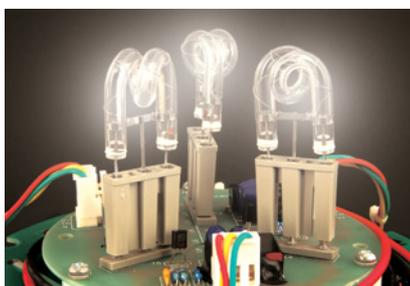
S180UHS type is a product that improves long distant visibility by equipping three high-intensity xenon lamps. The high performance product is typically used in harbors where there is fog, or mills/ steel mills where there is dust.
