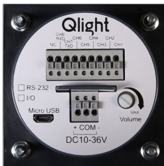
Terminal box for Signal phone panel(back side)
