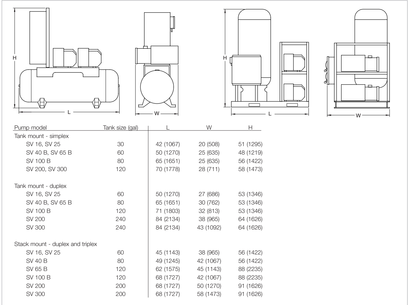
Central vacuum supply systems, tank mounted [left] and stack mounted [right]; dimensions in inch, dimensions in brackets ( ) are in mm
