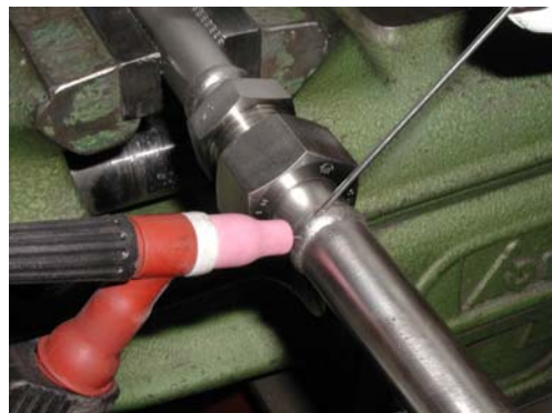
4. Unscrew the clamping nut and weld the tube connections. Pay attention to the negative pole
