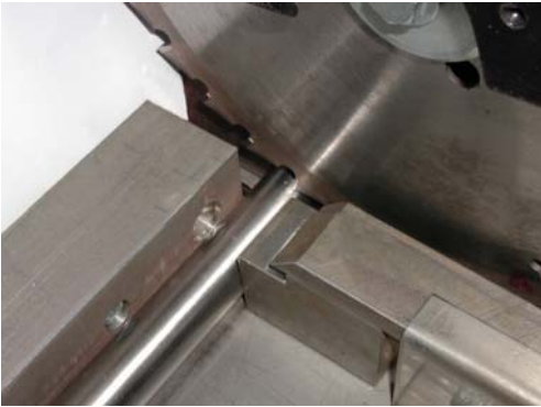
1. Saw off the tubes rectangularly
