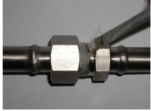
8. Lubricate – especially the austenitic steel - with suitable lubricants (e. g. type Never Seez from -180° C to +1400° C / order no. 05-1172-R001)
