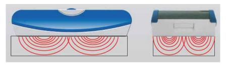
How it works: As soon as the sensor plate is in contact with the surface of the wood measuring starts.
