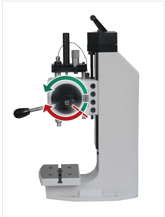
Return Stroke Lock Mode (the forward Stroke is released) Press blocks the return stroke when the necessary force has not been reached or the required stroke has not been reached. This ensures that the user always completes the operation.
