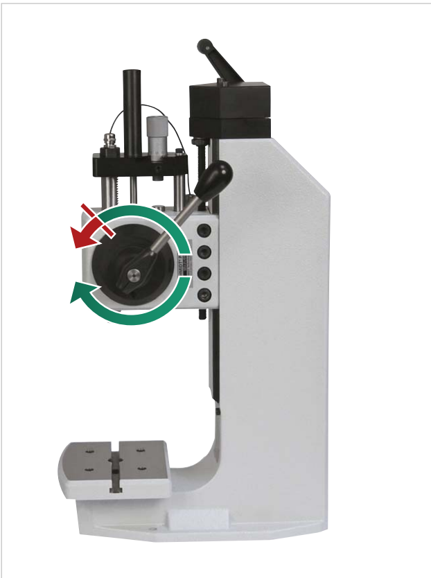
Forward Stroke Lock Mode (the return Stroke is released) For protecting the produced parts and the force sensor of the press the press blocked/restricts the force flow in forward stroke when reaching a defined force or when reaching the stroke.
