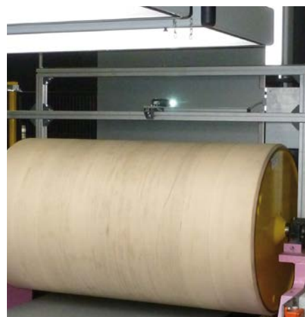
Color measurement of continuous strip coating such as aluminum, zinc and paper during production.
