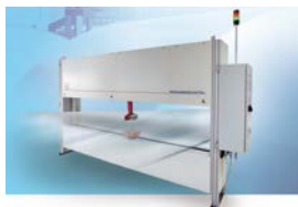
O-frame systems for profile thickness measurement thicknessCONTROL MTS 8201.LLT Page 14 - 15
