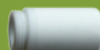
F5300 - Teflon (PTFE) sensor cover (white colour), with increased resistance against splashing water, non-absorbent surface, does not rust. Porous size 25µm. Temperature range -40°C to +125°C.
