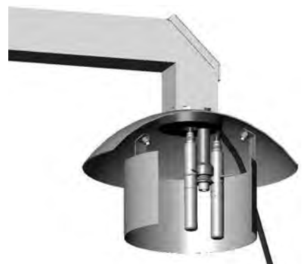
For calibration, a portable HMP77 reference probe is easy to attach beside HMT337 or PTU307 probe.
