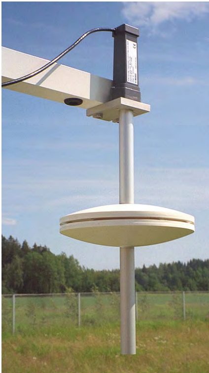
SPH10/20 is easy to install and connect. In the picture, SPH10 is connected to PTB210.
