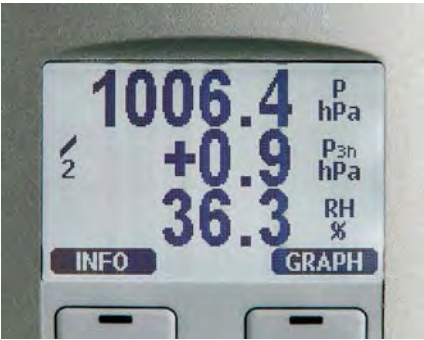
The display also shows the WMO pressure trend \Delta P_{3h} and tendency of 0 ... 8.
