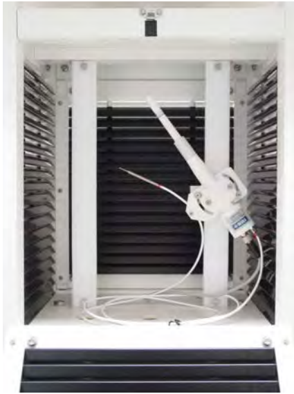
HMP155 with an additional temperature probe and optional Stevenson screen installation kit.
