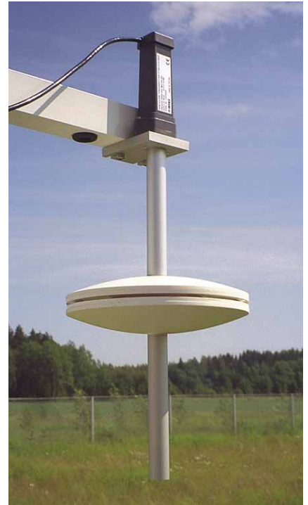
The SPH10/20 is easy to install and connect. In the picture, a SPH10 is connected to a PTB210 barometer.
