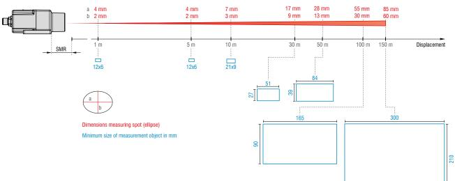
The ILR3800-100 sensor works with a semiconductor laser at a wavelength of 655 nm (visible/red). Laser power is <1 mW. The sensors fall within laser class 2. Devices of this laser class require no special safety precautions.
