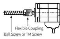
When connecting the load directly to the motor shaft, use a flexible coupling (ERB Series).
