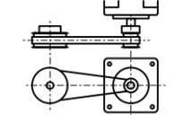
Connect the motor shaft and the line which connects the center of two pulleys to be perpendicular.
