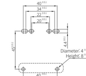
○ is installing spot of protrusion for fixing the switch firmly.
