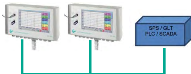
RS 485 network (Modbus RTU) or Ethernet (Modbus/TCP)
