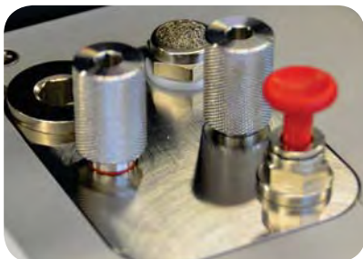
Sensor protected during transport or storage.
