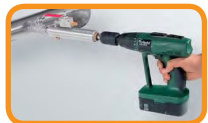
Drilling under pressure
